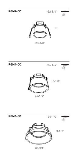
Every fixture includes a junction box with integrated dimmable driver Can be daisy chained Aluminum construction Switch-selectable CCT 40° beam angle 30° tilting, 360° rotation 5-year warranty
